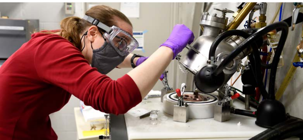
Postdoctoral Research Associate Lisa Pogue operates an arc melter in the McQueen Lab.
