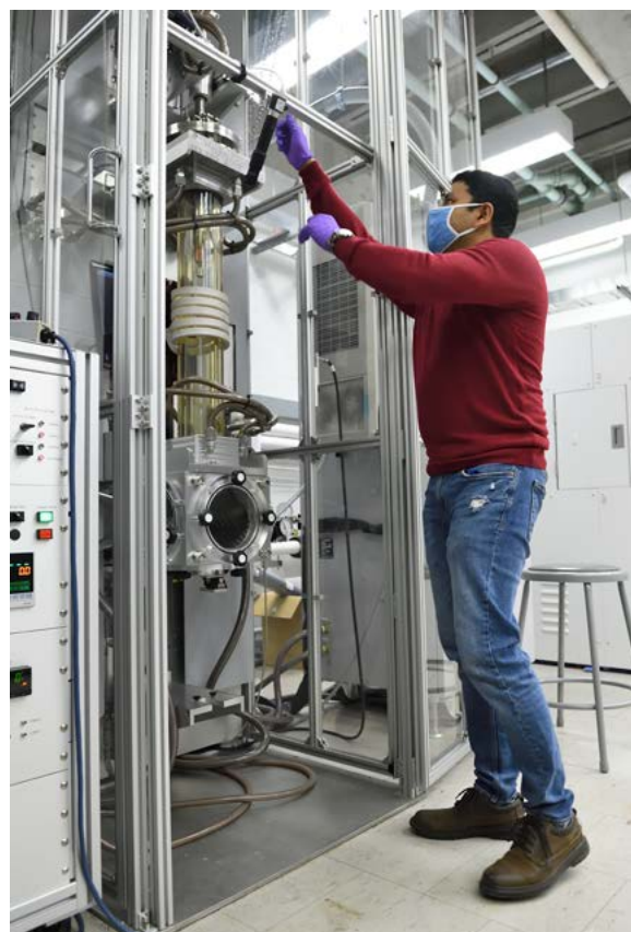
Mojammel Khan makes adjustments on an ultra high temperature induction furnace, a signature tool in the PARADIM lab.
