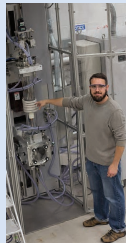
W. Adam Phelan, Ph.D., Associate Director of the PARADIM-Bulk Crystal Growth Facility, pictured with a radio frequency induction furnace.
