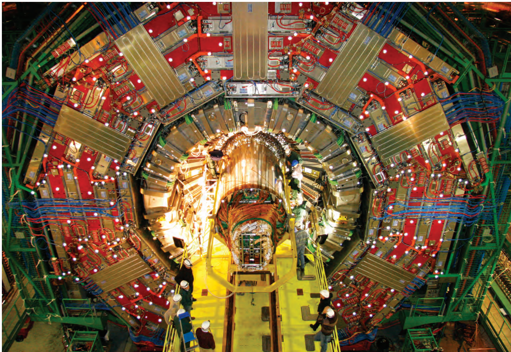
Installation of the CMS silicon tracking detector that Johns Hopkins researchers helped design, test, and install. (Photo courtesy of CERN)
